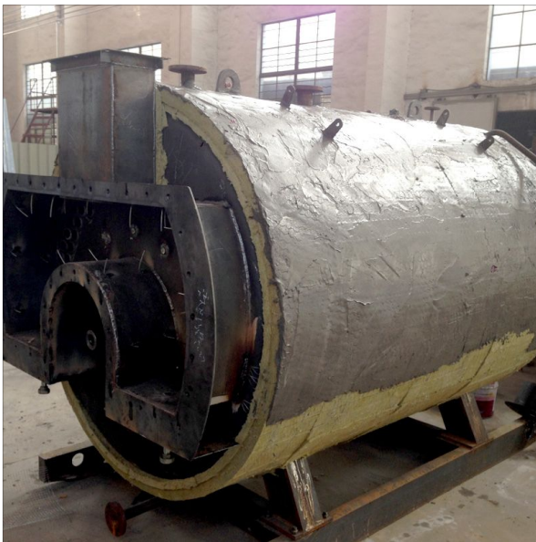
ZOZEN Boilers' Insulation Material 2. (Refractory cement on the rock wool)
